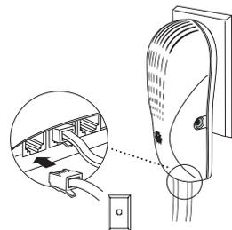
5. Connect the other end of the short telephone cable to a jack wired for a standard analog phone line.
